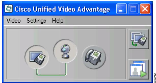
Figure 2-2 shows Cisco Unified Video Advantage associated with the Cisco Unified IP Phone. When Cisco Unified Video Advantage is connected to a Cisco Unified IP Phone, a solid green line connects the two buttons, and the buttons appear to be pressed.
